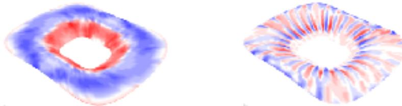
Fig 1. Utilization of the initial non-funicular shell (left) and a shell optimized with dynamic corrugation (right)
