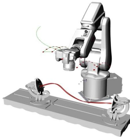
Figure 1: Photogrammetry reconstruction of a beam using a robotic arm.
