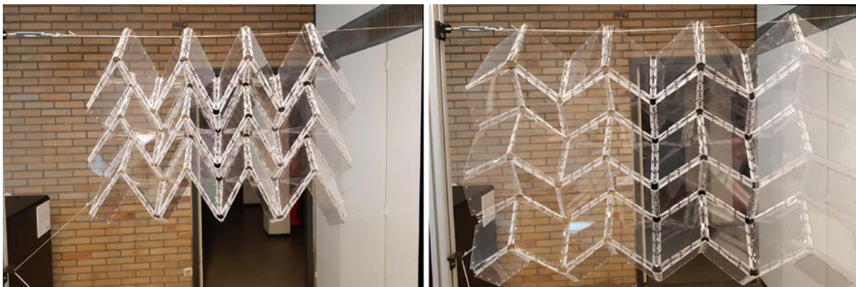
Figure 1: PALEO prototype made from 2mm polycarbonate with integral hinges, in two different deployment states
