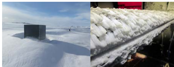
Figure 1: a) Snow deposition reference study in Nuuk, Greenland. b) Experimental icing in climatic wind-tunnel.
