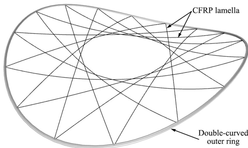
Figure 1: Single-layer crossover CFRP lamella cable-supported roof without inner ring
