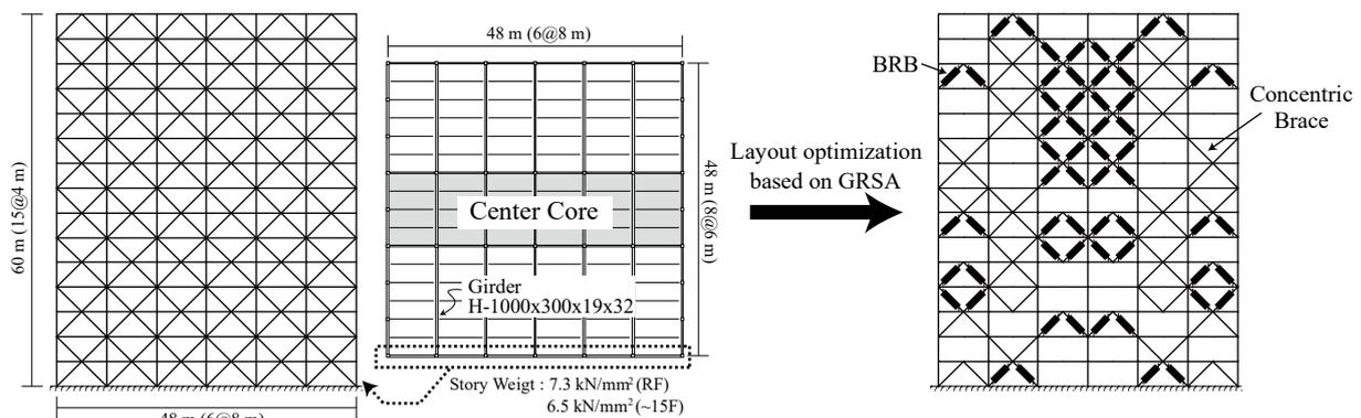
Fig. 1 Schematic image of the braced tubes.
