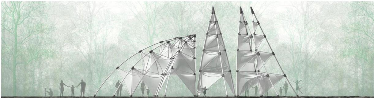
Fig. 1. Initial design of the pavilion with sliding mechanisms and actuation by support displacements
