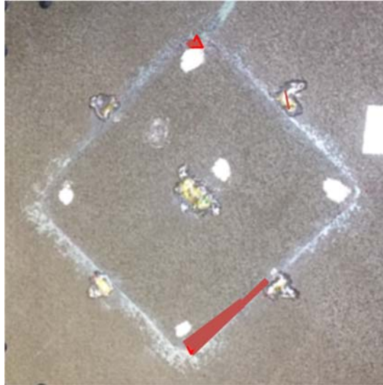
Figure 7. Ultrasonic inspection of repaired panel after shear testing.
