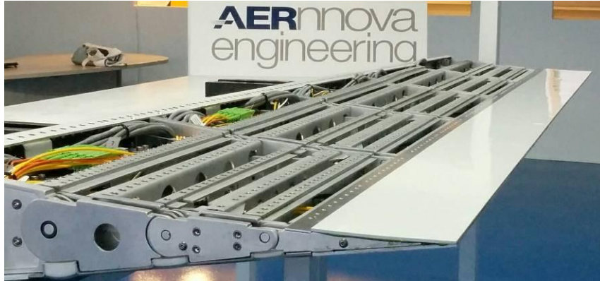
Figure 17: Internal structure of 5 Bay Demonstrator
