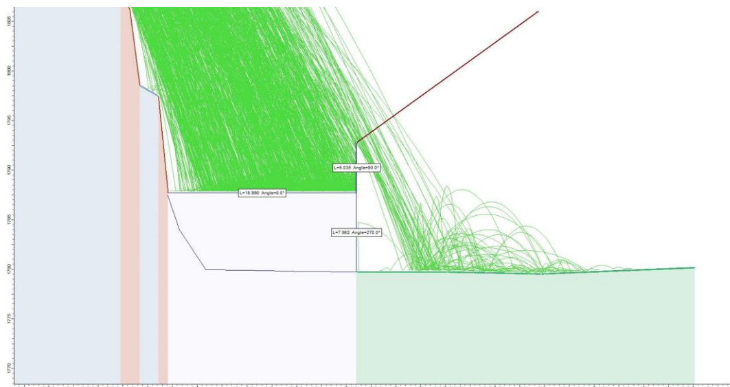
Fig. 3 Example results for final rockfall modelling showing the portal extension structure and flexible rockfall fence. Length of the extension was adjusted until 95% of the 1,000 blocks released were retained behind the barrier.
