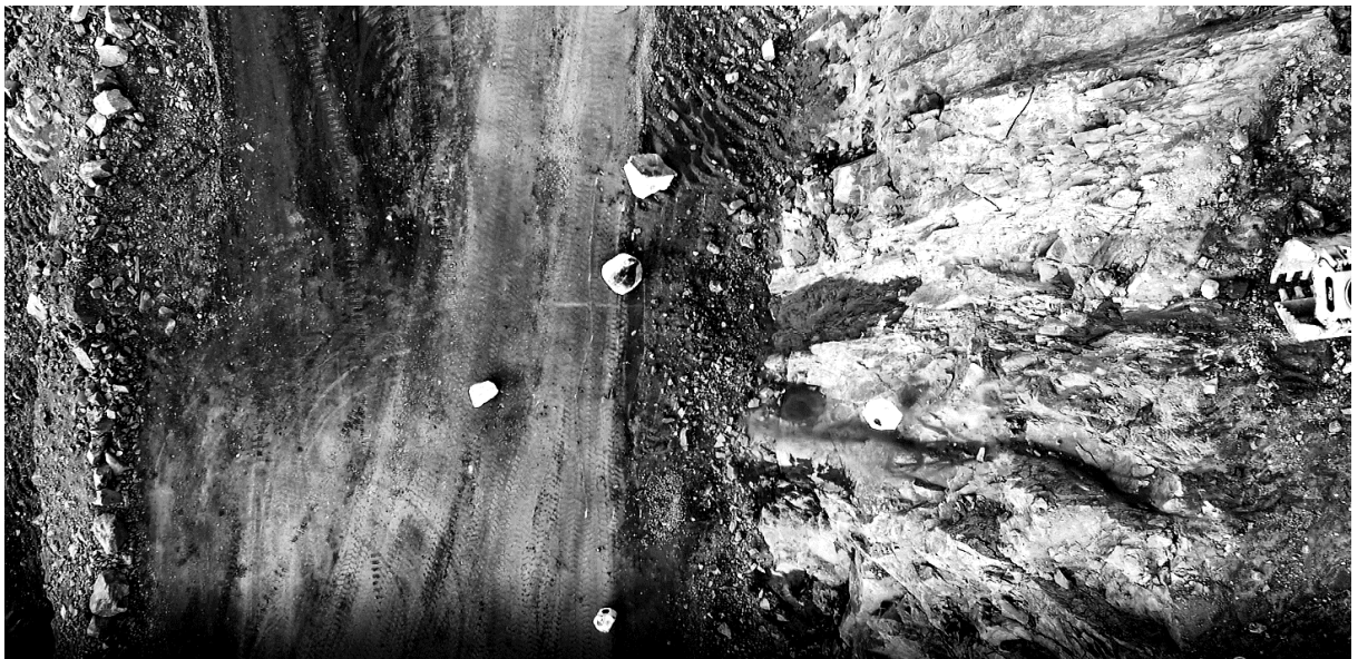
Fig. 2 Drop tests in a granite quarry at Limberg, Lower Austria. Geological unit of the Bohemian Massif. Monitoring with the aid of a video recording drone.
