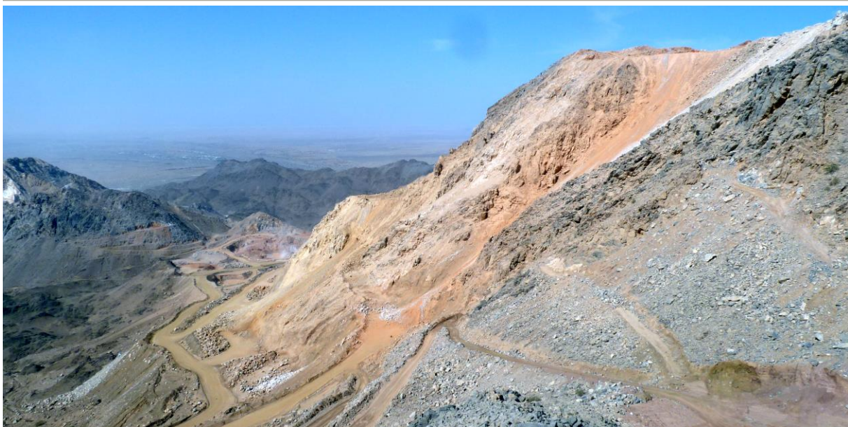
Fig. 1 View of the south side of the quarry mountain, with rock chute and accumulation areas.
