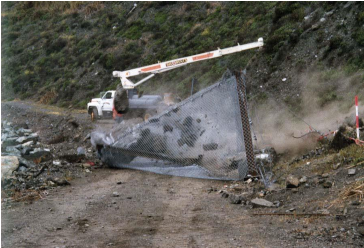
Figure 2: Flexible rockfall fence testing with different meshes and infrastructure configurations at the Shale Point test site in California, USA (Duffy & Hoon, 1996).
