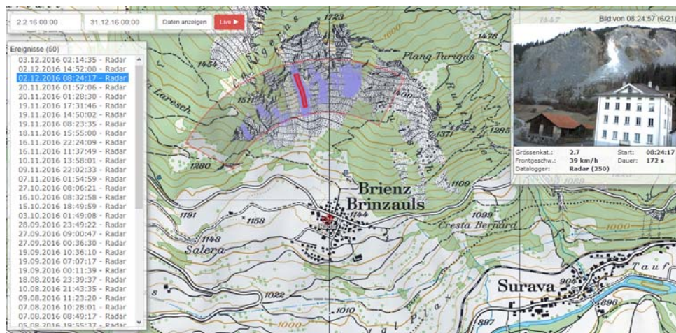
Fig. 4 All events are mapped immediately after detection on an online web portal. In addition, camera images are taken and uploaded automatically.
