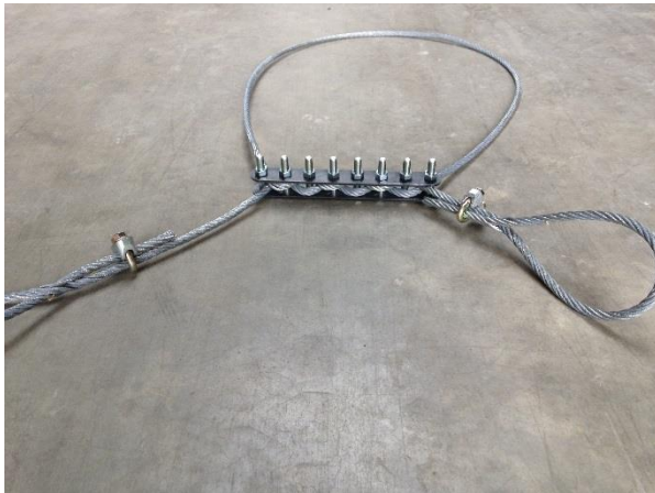
Fig. 4 GTS energy dissipating device and force-displacement results of the QS tensile tests.
