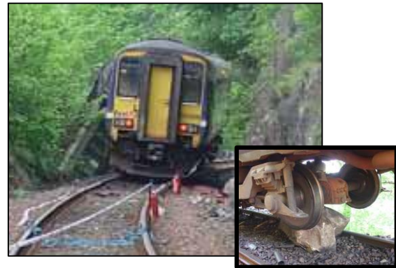
Fig. 2 Derailed train after collision with a fallen rock. [2]
