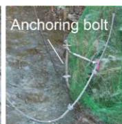
Photo 2 Failure of anchoring device (a: fracture, b: pull-out failure)
