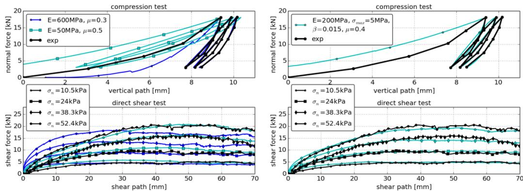
Figure 1: Comparison of experimental results of compression and direct shear tests to DEM simulations. Left: simplified Hertz-Mindlin model. Right: Conical Damage model. Experimental data taken from [1].
