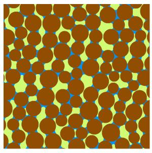
process governed by the increase of the liquid cluster volumes. Finally, we show that the evolution of capillary states is correctly captured by a simple model accounting for the competing effects of the Laplace pressure and grain-liquid interface.
