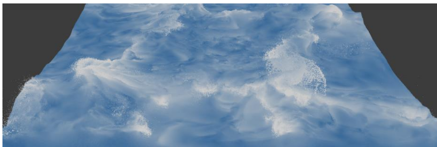
Figure 1: The neighbourhood search with compact hashing takes 22s on a 16-core PC in this breaking dam scenario with 107 million fluid particles.
