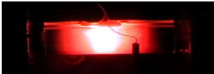
Fig.1. Melting process of the sample and visible no-uniform temperature distribution
