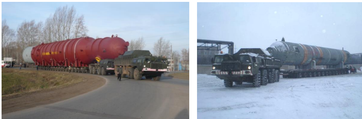
Figure 1: Typical multi-axis tractor-lorry-trailer combination intended for transportation of large-dimensioned indivisible loads
