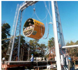
Figure 1: Drop test of a narrow-body Boeing-737 fuselage section [1]
