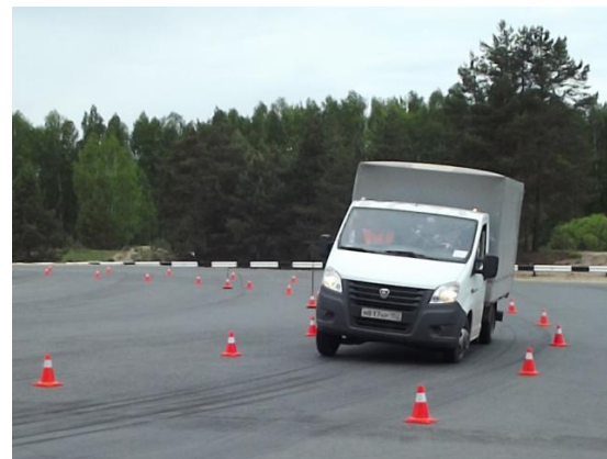
Figure 1: Experimental research (a – estimation of torsional stiffness of chassis frame in laboratory environment; b - estimation of critical speed for running into the corner maneuver)
