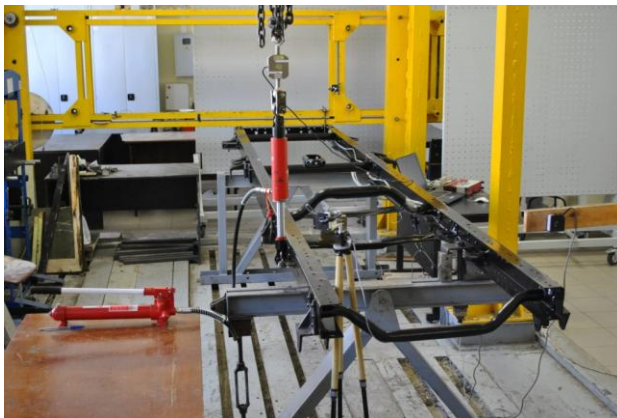
Figure 1: Experimental research (a – estimation of torsional stiffness of chassis frame in laboratory environment; b - estimation of critical speed for running into the corner maneuver)
