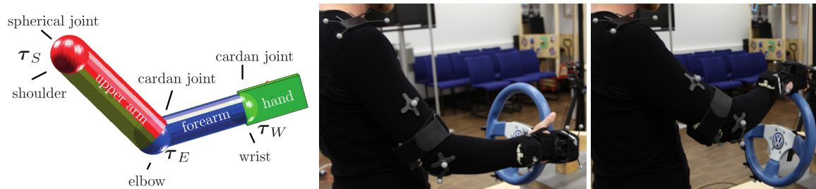
Figure 1: Left: human arm model used for optimal control simulations. Middle, right: Measurement setup showing the start and end position of the steering motion.
