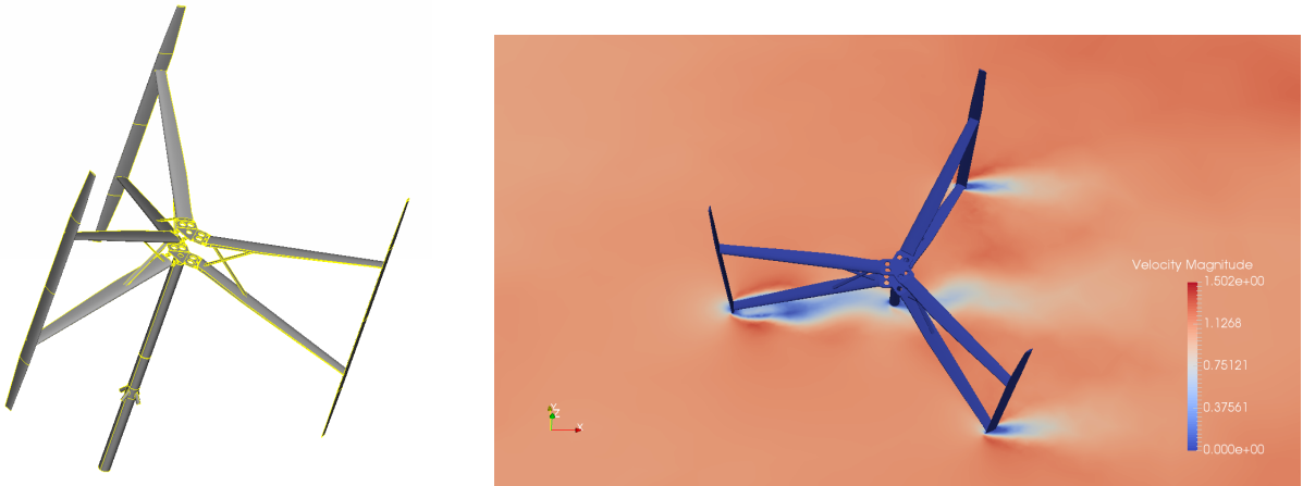
A vertical turbine (left) and a simulation of the flow past the rotating turbine (right).
