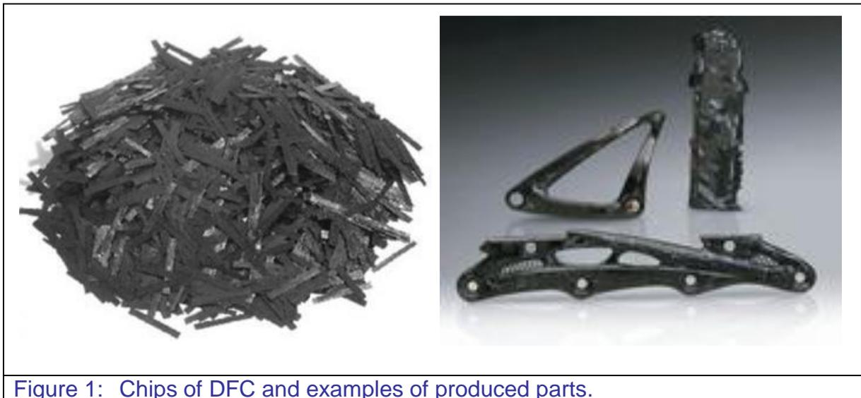
Figure 1: Chips of DFC and examples of produced parts.
