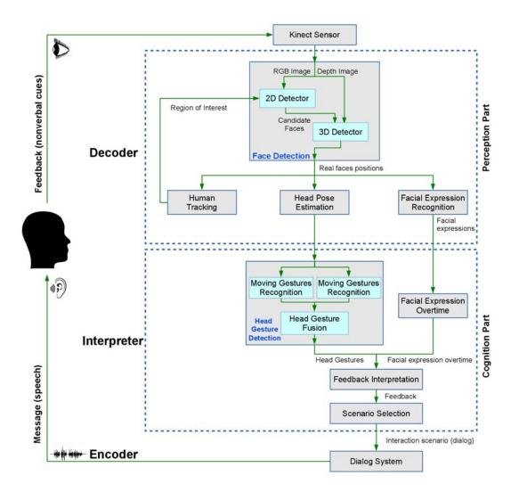
Figure 2: The proposed system overview. It consists of three modules: perception, cognition, and the dialog system. These three modules analogy to the decoder, interpreter, and encoder respectively.
