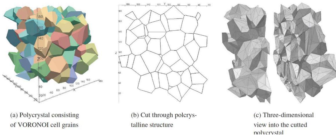
Figure 1: Polycrystal and discretization
