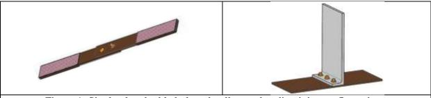
Figure 1: Single –lap double bolt and pull out + bending joint configurations
