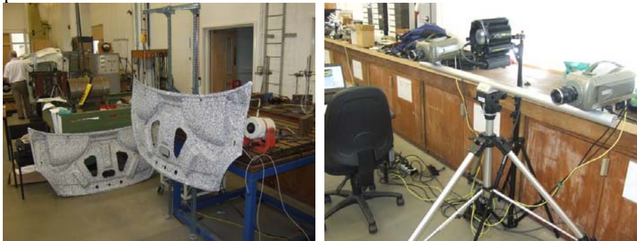
Figure 1: Setup of High Speed DIC system (right) and bonnet structure with shaker (left)
