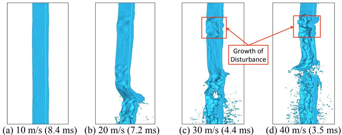
Fig.1 The deformation of liquid sheet at early stage
