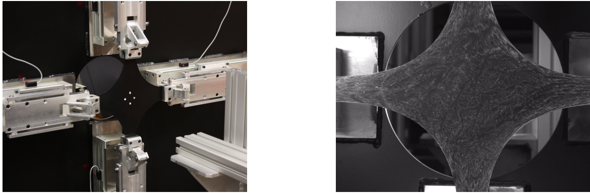
Fig. 1 : Experimental equipments for non proportional loading, biaxial tension
