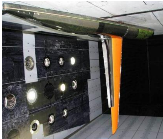
Figure 2: DLR-F11-DS21 model mounted in ETW wind tunnel
