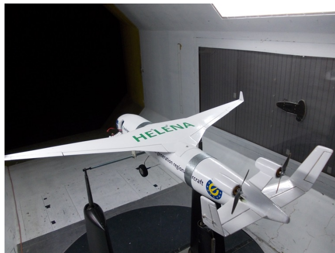
Fig. 1 – Wind tunnel model w/ active smart wing
