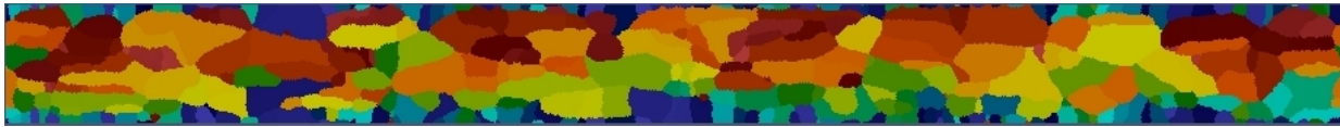
Figure1. Final microstructure obtained after complete phase transformation during heating. Different colours represent different austenite grains.
