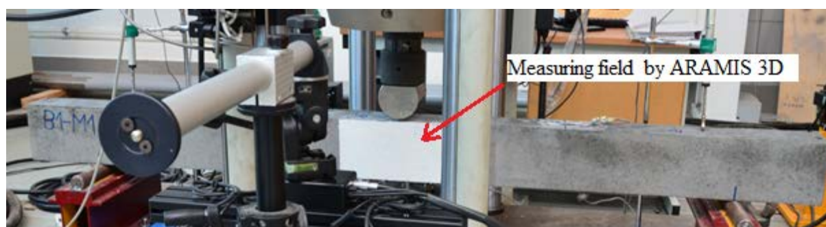
Figure 1: Testing machine (three-point bending test) and monitoring of damage zone by ARAMIS 3D
