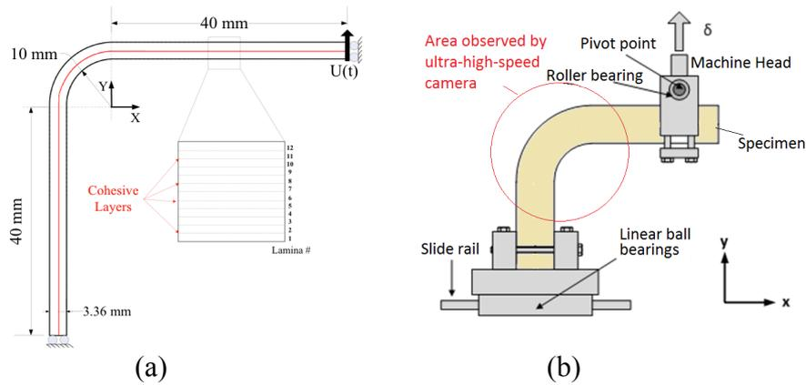
Fig. 1 (a) L-shaped composite specimen dimensions, boundary conditions and the location of cohesive elements for the numerical study and (b) experimental set-up.
