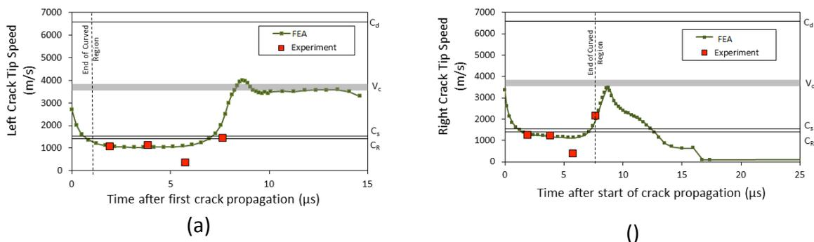
Fig. 3 Crack tip speed as a function of time graphs obtained by FEA and experiments for (a) left and (b) right crack tip speeds.
