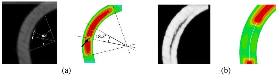
Fig. 2 Experimental high-speed photo and finite element snapshot of normal stress contours at (a) instant of delamination initiation and (b) during delamination propagation.
