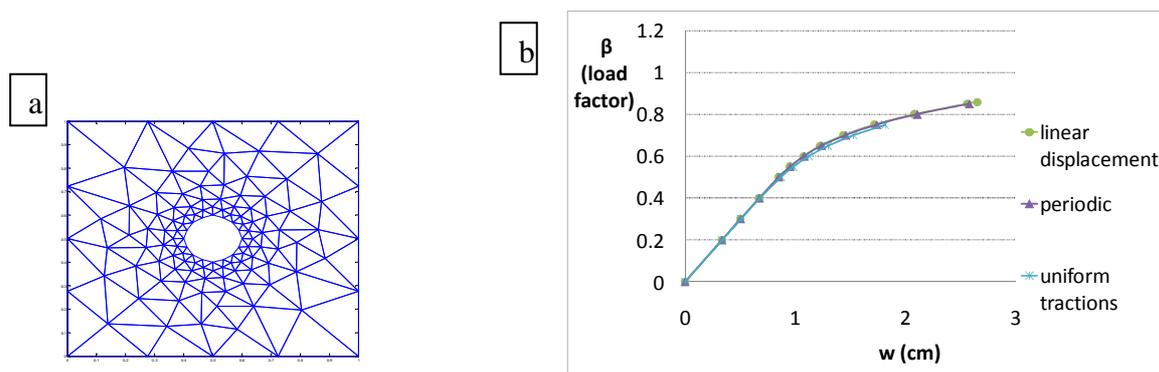
Figure 2 – a)Discretization of a RVE with a void defined in the centre b)Deflection at the central point of the beam, using different boundary conditions in the RVE
