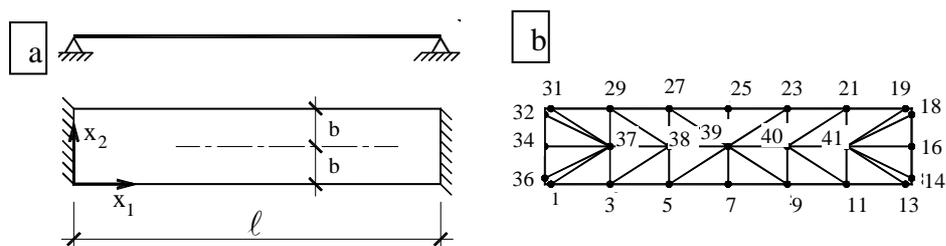
Figure 1 – Simply supported beam – geometry and discretization
