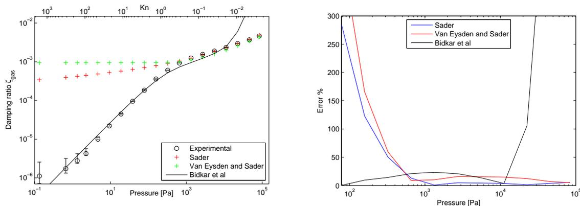
Figure 1: Comparison of the predictions of the Sader’s model [1], Van Eysden and Sader’s model [3] and the ES-BGK-model-based fit, with the experimental gas damping values for microcantilever A in its first mode [4]. a) Damping ratio values, b) relative percent error.
