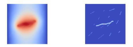
Figure 1: Fluid driven fracture in the presence of natural fractures. Note crack turning, intersecting, and being influenced by the presence of natural fractures. Contours of pressure are shown on the left and contours of damage are shown on the right.
