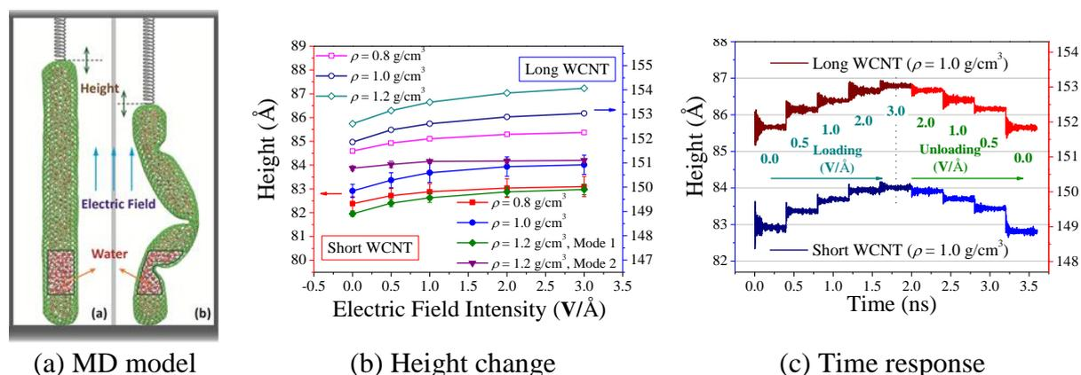
Fig.2 The deformation response of water-filled CNTs
