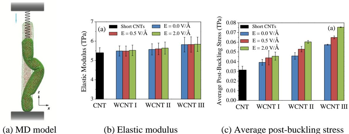
Fig.1 The mechanical property of water-filled CNTs
