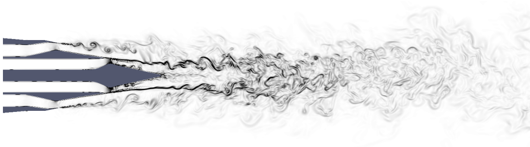
Figure 1: The density-field gradient contours of the high subsonic jet exhausting a coaxial nozzle is shown.
