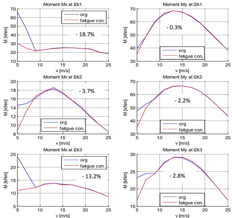
Figure 4: Equiv. load range for damage exponents  $m = 3$ , baseline control (blue) and advance control (red)
