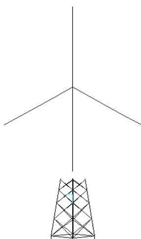
Figure 1: Offshore wind turbine beam model (HAWC2)
