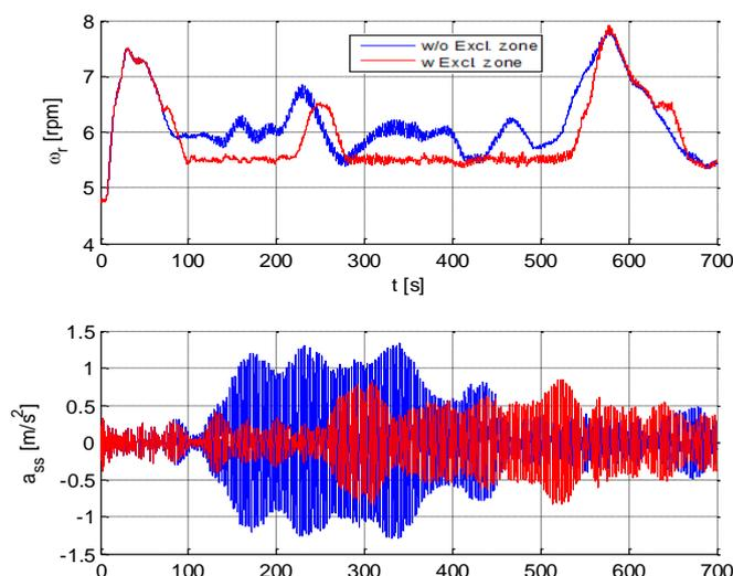
Figure 2: Exclusion zone – rotor speed (up) and tower side to side acceleration time responses (down)
