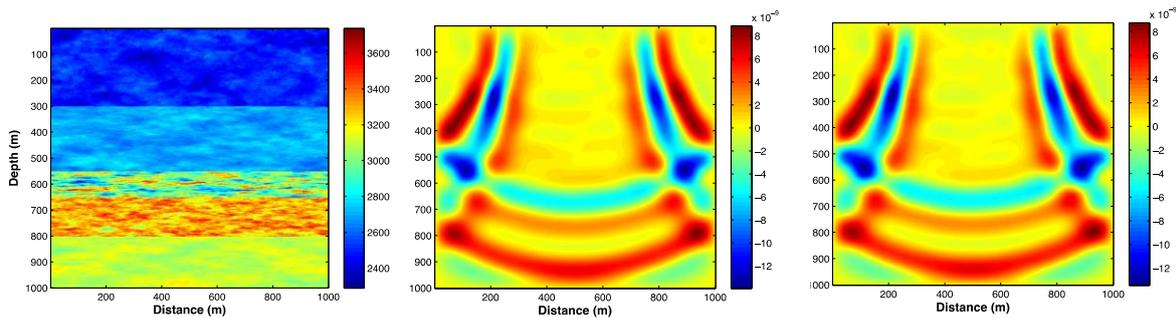
**Fig. 1:** Left: earth model with acoustic wave velocity in m/s; center: fine-scale reference solution at propagation time 0.4 s ; right: representative multiscale solution at time 0.4 s.
