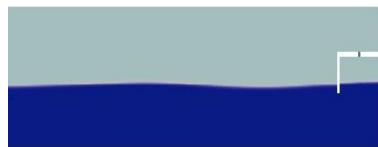
Figure 1: Snapshot of the domain used for the simulations: the waves are generated in the left part; the confined space on the right part represents the air chamber, while the small orifice mimics the turbine inlet nozzle. No-slip condition were applied to the boundaries that had to be considered solid, while Neumann and Convective BC were tested on the free boundaries.
