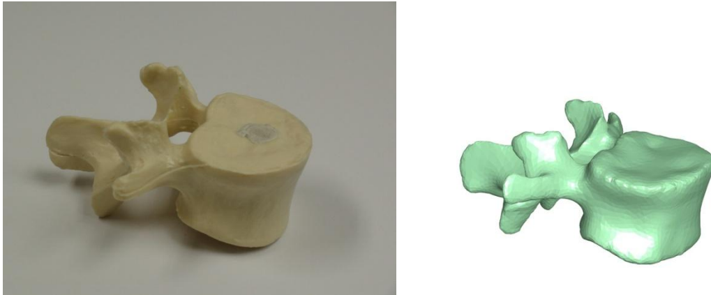
Fig. 1 STL geometry obtained with 3d scanner
