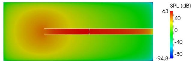
**Figure 1:** Distribution of Sound Pressure Level SPL [dB] in computation domain
