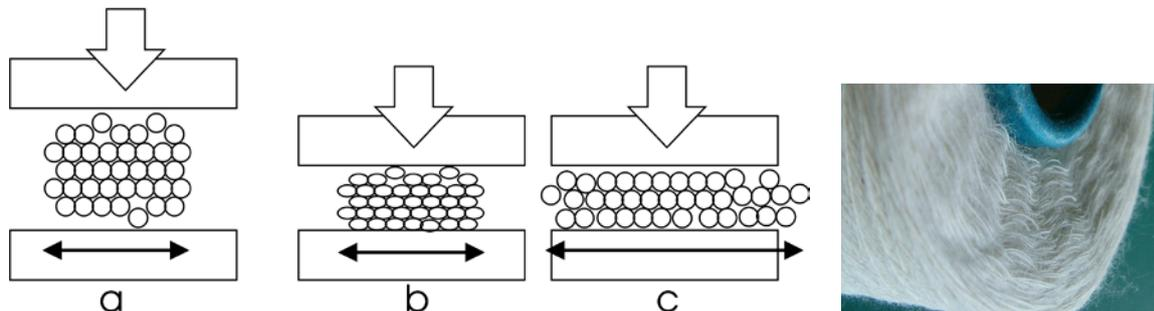
Figure 2. Changes of the yarn cross section a) initial cross section of multifilament yarn, b) deformed cross section of compressible yarn c) "deformed" or more precisely rearranged cross section of incompressible yarn d) compressed windings inside of the bobbin as result of not correct chosen winding tension.
