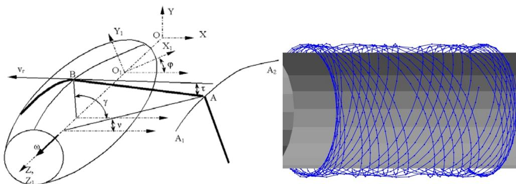
Figure 1. General geometry of the winding process following [4]. The yarn guide A is moving along the curve  $A_1A_2$ , the winding point B is the current first fixed point of the yarn over the bobbin surface. The bobbin rotate with angular velocity  $\omega$  ; b) simulated yarn path during the winding
