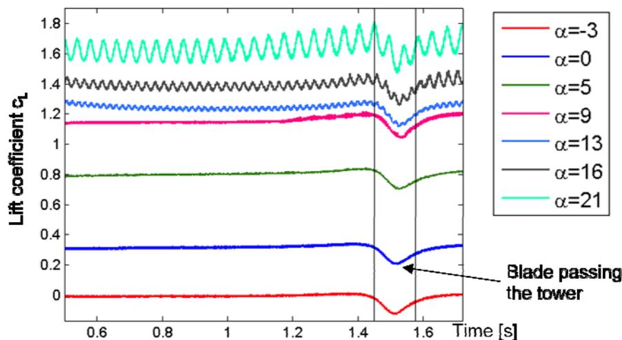
Fig. 1: Lift coefficients of blade profile depending on pitch angle  $\alpha$ .
