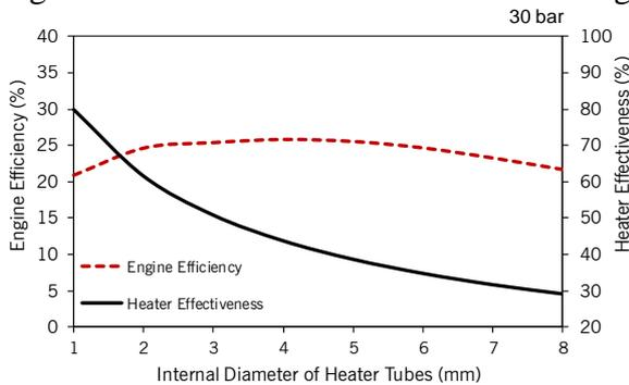
**Figure 2.** Engine efficiency and heater effectiveness as a function of the internal diameter of the heater tubes.
