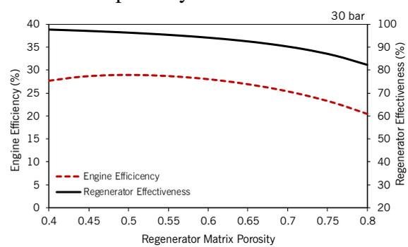
**Figure 3.** Engine efficiency and regenerator effectiveness as a function of the regenerator matrix porosity.
