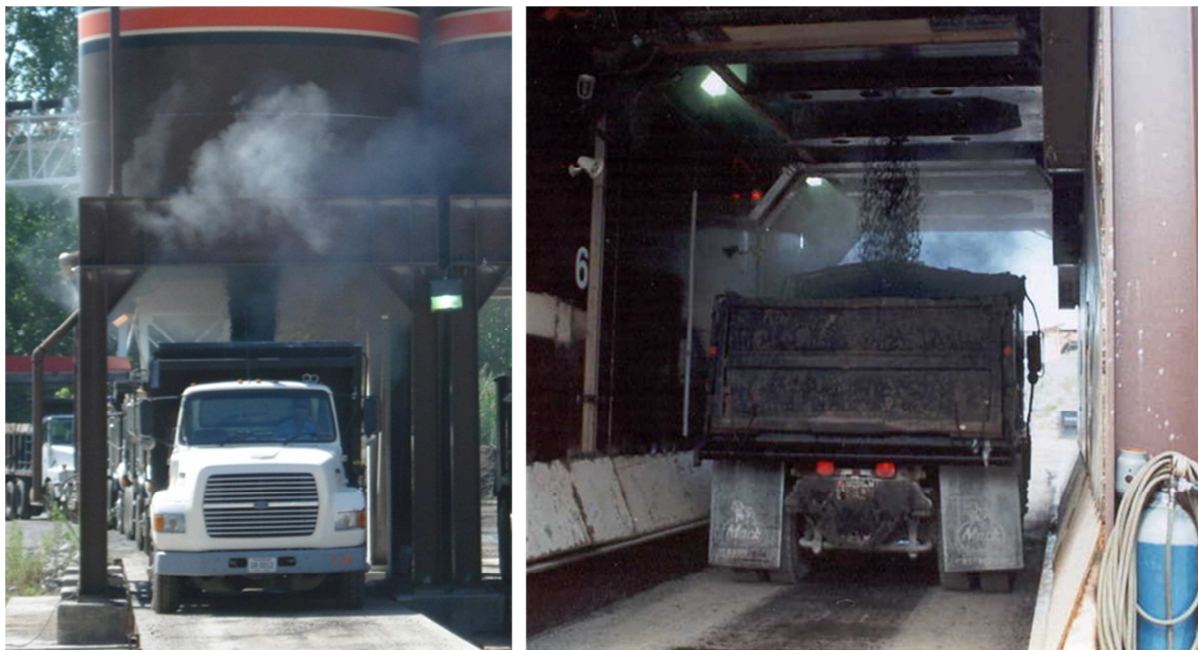
Figure 1. Silo to truck transfer showing smoke formation
