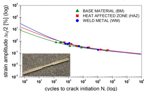
**Figure 2:** Strain-life of the three zones BM, HAZ and WM for a S960QL butt weld (preliminary results)
