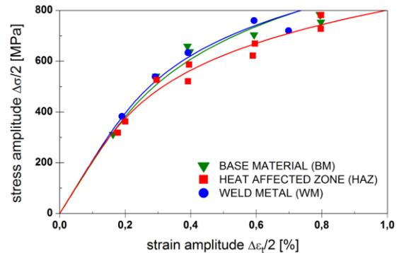
**Figure 3:** Cyclic stress-strain relation of the three zones BM, HAZ and WM for a S960QL butt weld (preliminary results)
