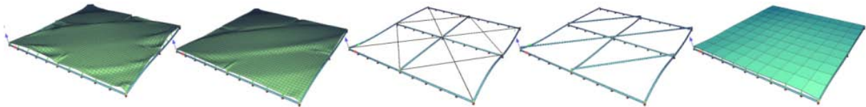
Figure 5: Deformation of 4-field grid restrained with membranes with E = 500 \text{ N/mm}^2 and E = 2000 \text{ N/mm}^2 (exaggerated by a factor of 2), diagonal cables, bars and plywood panels (exaggerated by a factor of 5) under a horizontal load of 1.15 kN at Point A
