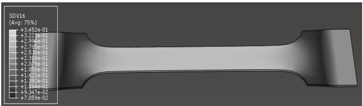
Figure 3: Simulation results of the energy storage rate for a steel
