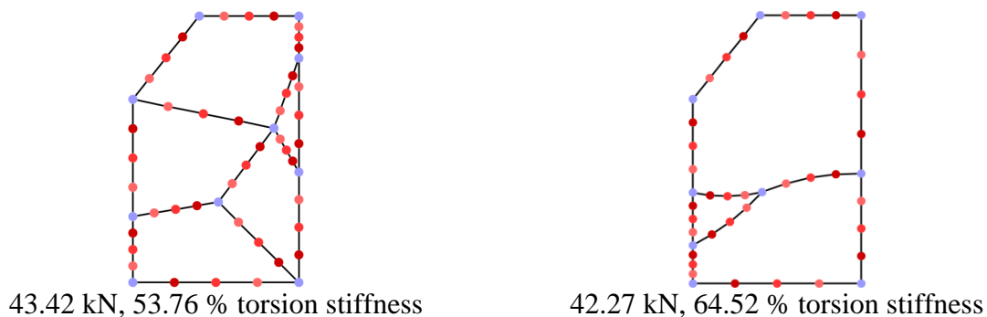
Figure 9: Graphs of the final designs generated without (left) / with (right) the usage of competing designs
