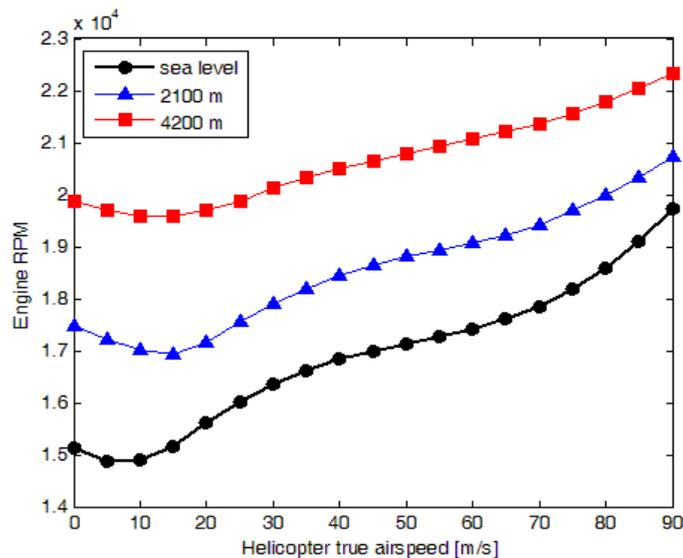
**Figure 1.** Engine RPM corresponding to optimal main rotor speed for different helicopter flight conditions.
