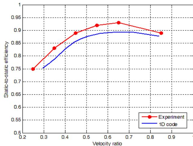
**Figure 5.** Validation of TDES code upon single stage B.
