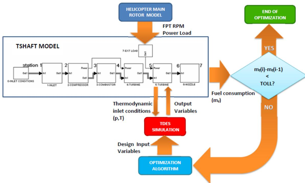
**Figure 6.** FPT redesign optimization procedure.
