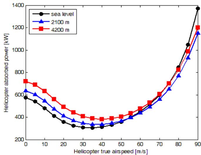
**Figure 2.** Helicopter absorbed power at optimal main rotor speed for different helicopter flight conditions.
