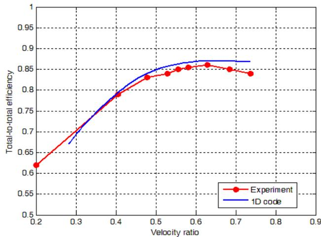
**Figure 4.** Validation of TDES code upon single stage A.
