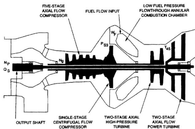
**Figure 3.** Cross section of a GE T700 turboshaft engine [18].
