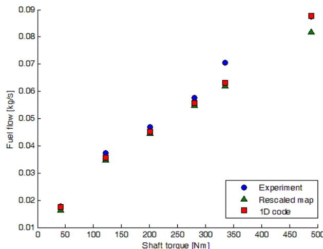
**Figure 7.** TSHAFT engine model validation coupled with TDES model: fuel flow comparison with experimental data and rescaled characteristic map.
